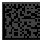
Figure 3.6.1.2-1 A symbol with very poor Symbol Contrast.
