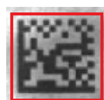
Figure 3.6.2-6 Quiet Zones of a Data Matrix
